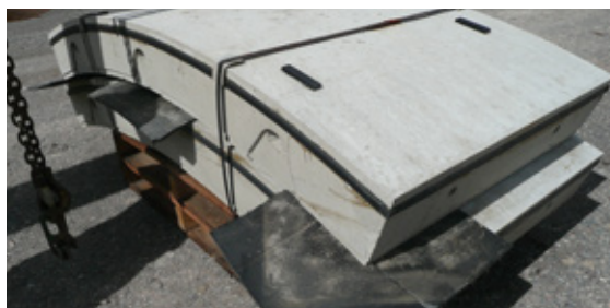
Top: Rubber mats placed between the two segments
